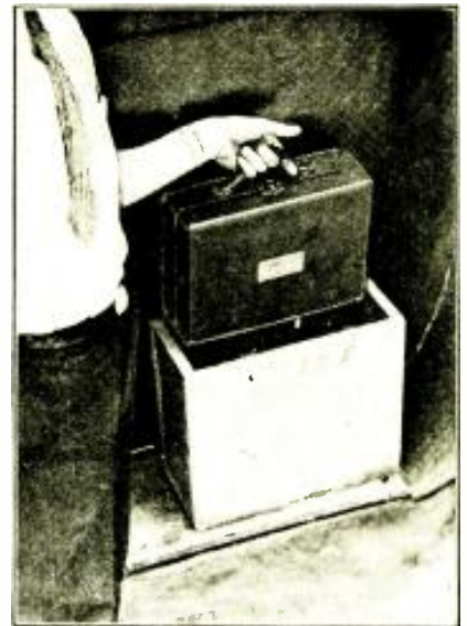
A high-grade meter deserves to be handled with care; and a shockproof container like this is desirable.
