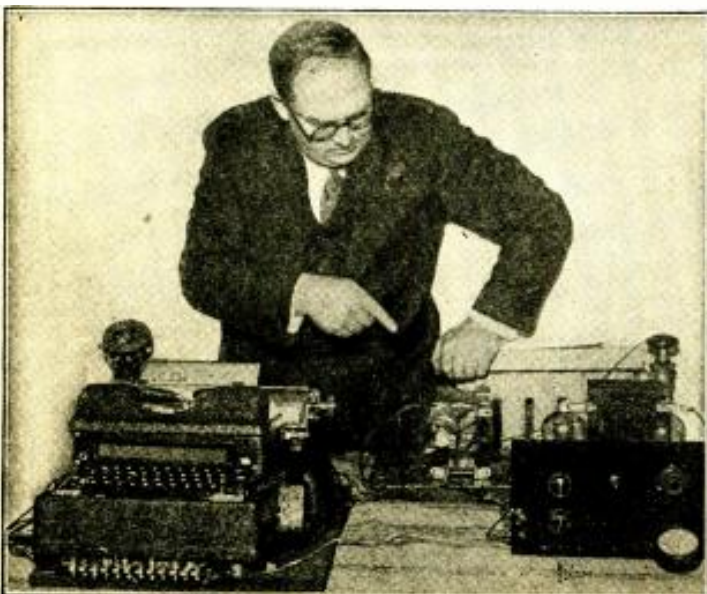
Fig. B (left) The receiving typewriter at the left, with its short-wave receiver at the right. The latter is standard. The machine has a commutator rotating in exact synchronism with that of the transmitter.
